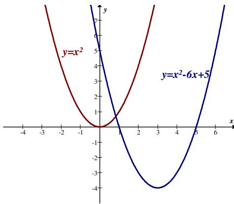
$$\begin{aligned} f(x) &= x^2 - 6x + 5 \\ &= x^2 - 2 \cdot 3x + 9 - 9 + 5 \\ &= (x - 3)^2 - 4 \end{aligned}$$
